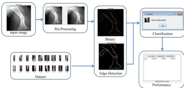
**Fig-2 :** Flow Diagram
